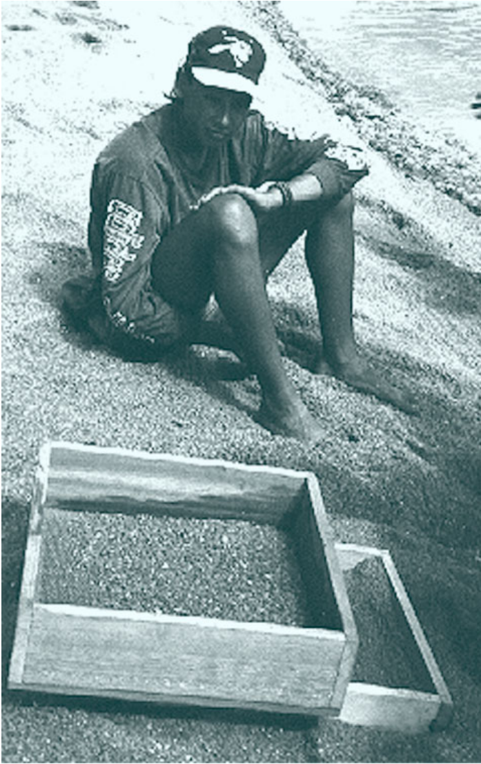
Figure 16.6 For sand from coarse grained areas, a larger sieve needs to be used. (Photograph Geoff Jensen)
