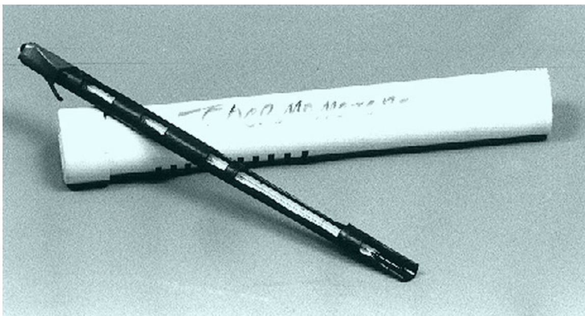
Figure 47.7 Home made field thermometer. A number can be stored in some sink drain pipe with a cap at each end.
