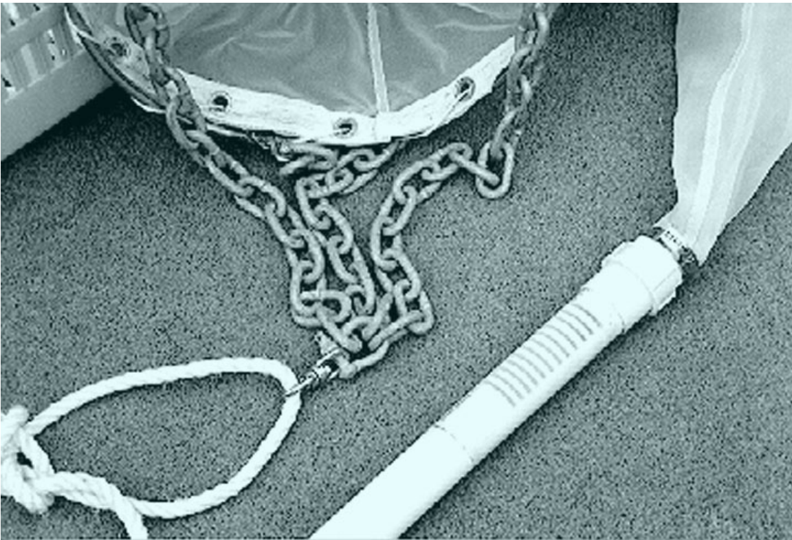
Figure 46.3 A more expensive home made plankton net: close-up of key elements (Wet Paper design)
