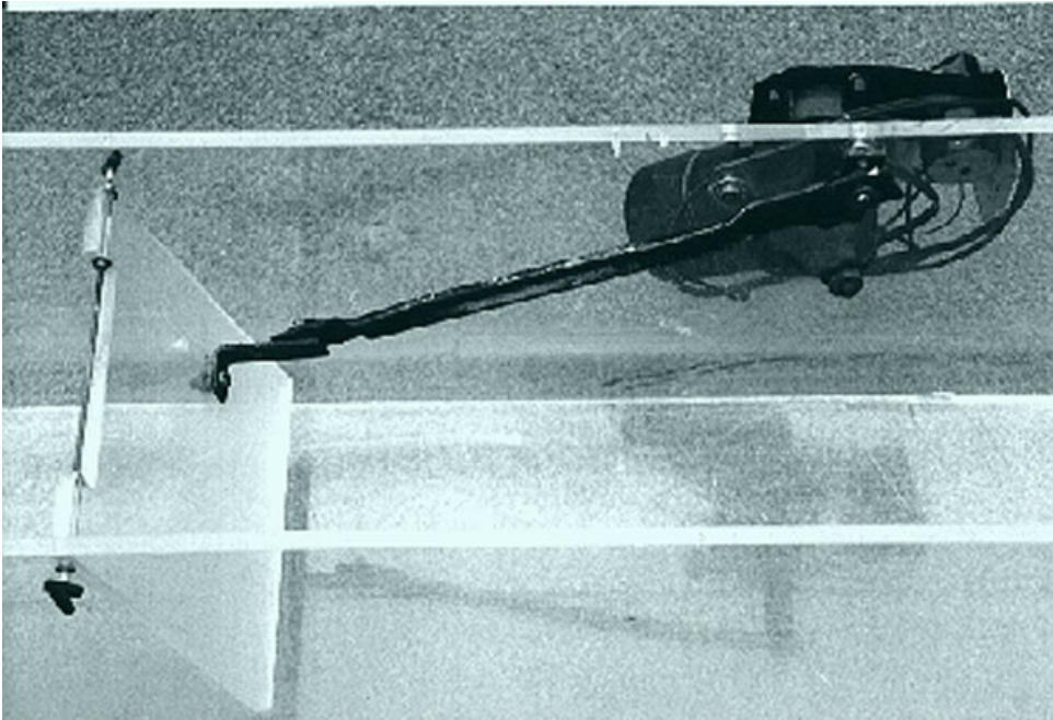
Figure 15.4 Close up of wave paddle setup
